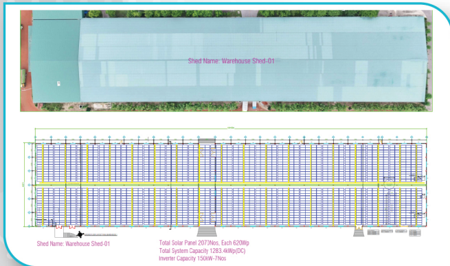
Autocad Design-Industrial Shed
